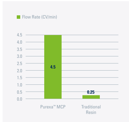
Figure 3. Purexa™ MCP is able to function at 22 times faster flow rates compared to tradition resin products with 10 times higher binding capacity.
